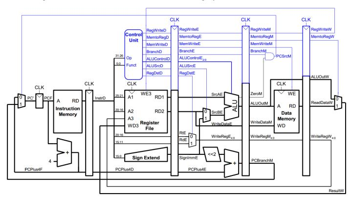
A pipeline hazard occurs when an instruction depends on result from a previous instruction that hasn't completed; this can be either a data hazard when the register value hasn't been written back yet or a control hazard where the next instruction is not yet decided (caused by branches).
