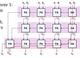
Multipliers (pictured) are the largest common arithmetic block and consists of three parts: partial product
